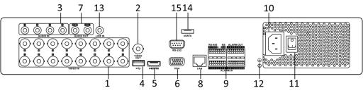
Figure 1-15 Rear Panel of DS-7300HQHI-K (with 16 Video Inputs)
