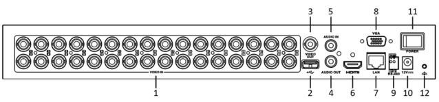
Figure 1-24 Rear Panel of DS-7200HGHI-K2
