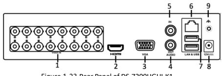
Figure 1-23 Rear Panel of DS-7200HGHI-K1
