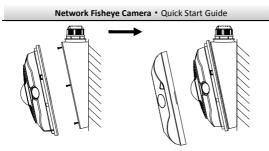
Figure 2-7 Install the Camera Body and Cover
