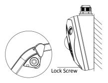
Figure 2-8 Tighten the Lock Screw on the Camera Cover
