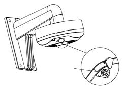
Figure 2-14 Tighten the Screw on the Camera Cover
