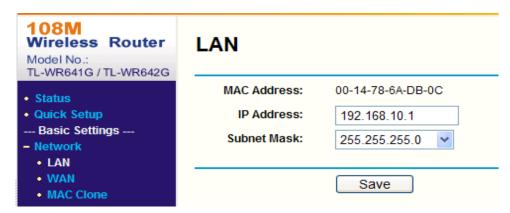
Figure A.2.2 Set the LAN parameters
