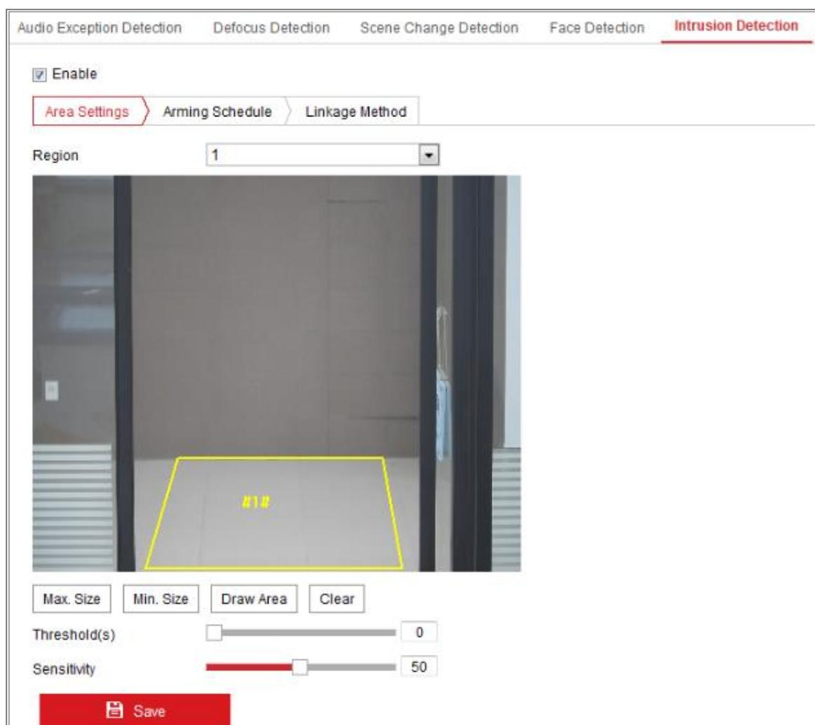
Figure 10-19 Intrusion Detection
