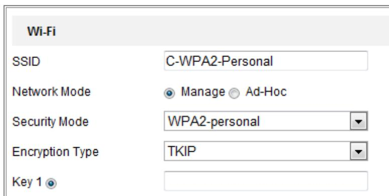
The screenshot shows a 'Wi-Fi' settings panel. The 'SSID' field contains 'C-WPA2-Personal'. Under 'Network Mode', the 'Manage' radio button is selected, and 'Ad-Hoc' is unselected. The 'Security Mode' dropdown is set to 'WPA2-personal', and the 'Encryption Type' dropdown is set to 'TKIP'. The 'Key 1' radio button is selected, and its corresponding text input field is empty.
