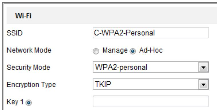
The screenshot shows the same 'Wi-Fi' settings panel as Figure 4-2, but with the 'Ad-Hoc' radio button selected under 'Network Mode'. The 'Manage' radio button is now unselected. All other settings (SSID, Security Mode, Encryption Type, and Key 1) remain the same as in the previous figure.
