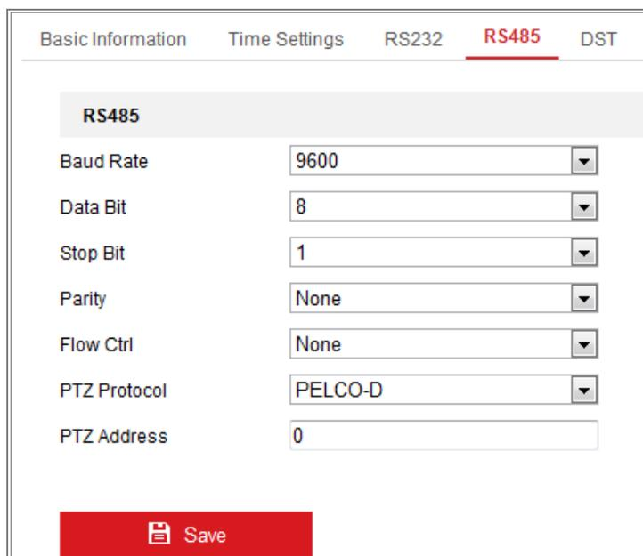
The screenshot shows a web-based configuration interface for RS485 settings. At the top, there are tabs for 'Basic Information', 'Time Settings', 'RS232', 'RS485' (which is selected and highlighted in red), and 'DST'. Below the tabs, the 'RS485' section is displayed with the following parameters and their values:
