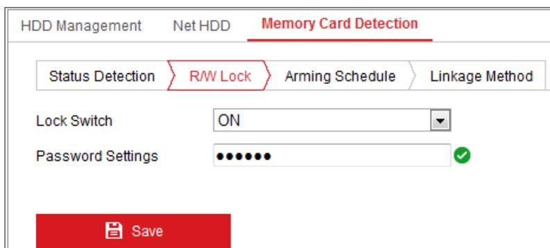
The screenshot shows the 'Memory Card Detection' configuration page. At the top, there are tabs for 'HDD Management', 'Net HDD', and 'Memory Card Detection'. Below the tabs is a navigation bar with four items: 'Status Detection', 'R/W Lock' (highlighted with a red box), 'Arming Schedule', and 'Linkage Method'. The main content area has two settings: 'Lock Switch' set to 'ON' and 'Password Settings' with a masked password field and a green checkmark. A red 'Save' button is at the bottom.
