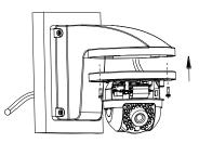
(6) Install the housing and lock the screws. (7) Finish the installation.
