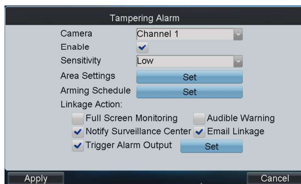
Figure 4.26 Set Video Tampering Alarm
