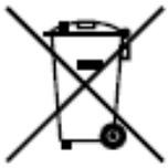
2006/66/EC (battery directive): This product contains a battery that cannot be disposed of as unsorted municipal waste in the European Union. See the product documentation for specific battery information. The battery is marked with this symbol, which may include lettering to indicate cadmium (Cd), lead (Pb), or mercury (Hg). For proper recycling, return the battery to your supplier or to a designated
