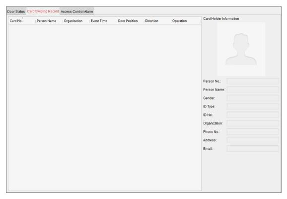
The logs of card swiping records of all access control devices will display in real time. You can view the details of the card swiping event, including card No., person name, organization, event time, etc.
