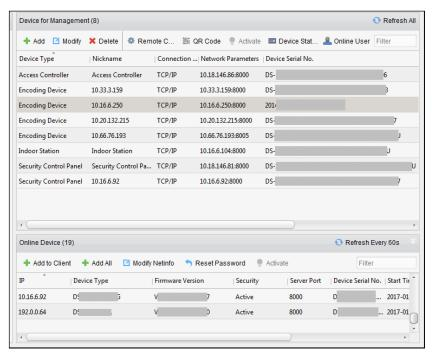
**Note:** After adding the device, you should check the device arming status in **Tool** – **Device Arming Control**. If the device is not armed, you should arm it, or you will not receive the real-time events via the client software. For details about device arming control, refer *7.13 Arming Control*.
