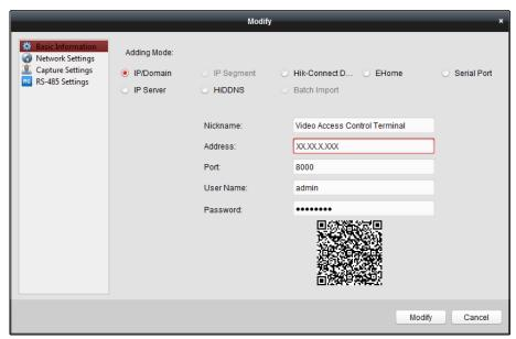
4. Edit the device information, including the adding mode, the device name, the device IP address, port No., user name, and the password.
