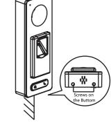
6. Tighten the screws on the bottom of the terminal to fix the terminal on the mounting plate and complete the installation.
