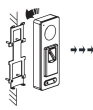
5. Push the terminal in the mounting plate from bottom up.
