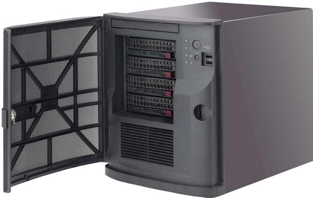
The DIVAR IP all-in-one 5000 appliance is an affordable and easy to use all-in-one recording, viewing, and management solution for network surveillance systems of up to 42 channels (with 8 channels pre-licensed).
