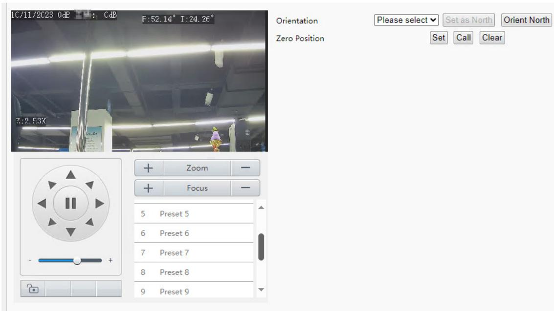
2. Select the mode to calibrate the camera to north.
