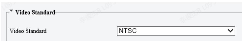
3. Select the P/N standard from the **Video Standard** drop-down list. Even if you switch the capture mode in [Video](#), the P/N standard configured in this page still prevails.
