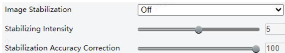
2. Select **On** or **Off** to enable or disable image stabilization, and configure the parameters.
