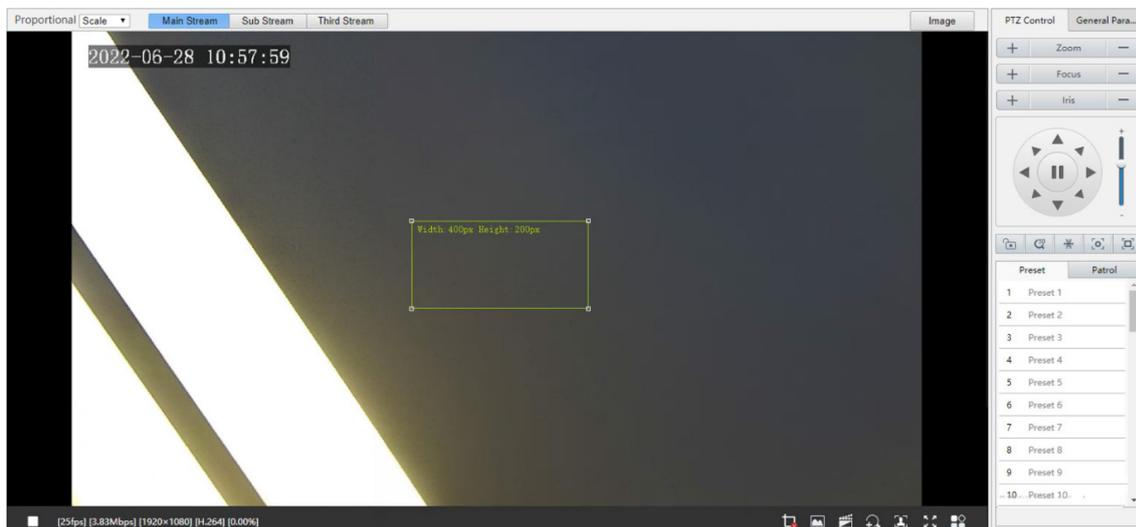
2. Adjust the position and size of the detection area. The pixel value changes with the size of the detection area.
