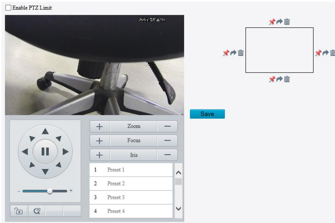
2. Set the pan and tilt limits. Take the tilt limit configuration as an example:
