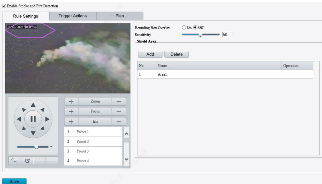
(3) Adjust the position and size of the area or draw an area as needed.
