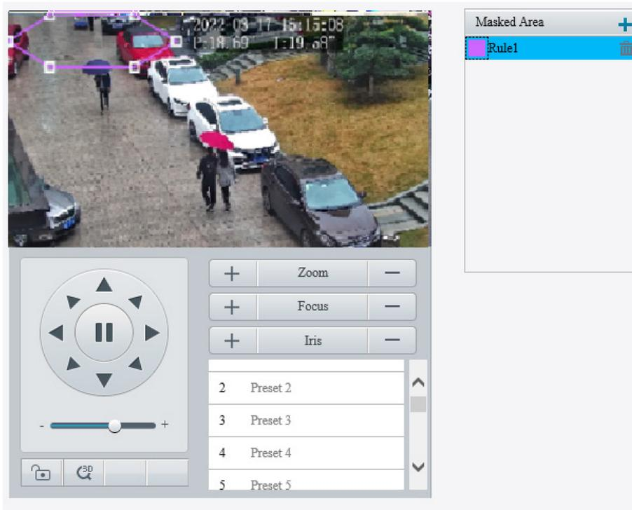
(2) Adjust the position and size of the area or draw an area as needed.
