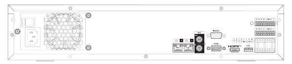
The NVR44-16P-4KS2/NVR44-16P-4KS2/L/NVR44-16P-4KS2/I series rear panel is shown as below.
