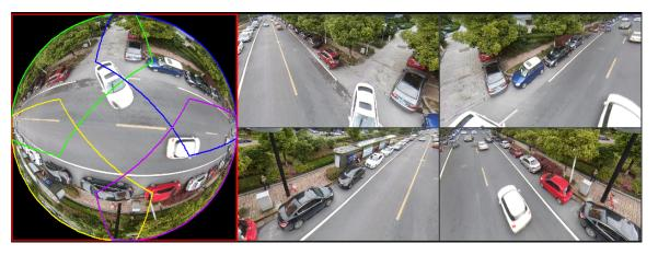
You can adjust the color pane on the left pane or use your mouse to change the position of the small images on the right pane to realize fish eye de-warp.
