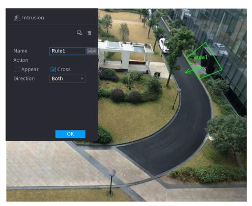
Figure 5-127 Intrusion (AI by camera)
