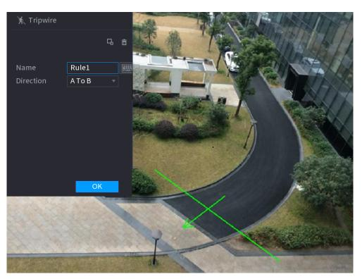
Figure 5-123 Tripwire (AI by camera)
