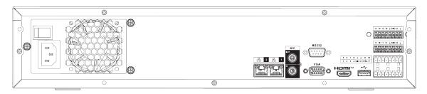
The NVR48-16P-4KS2/NVR48-16P-4KS2/L/NVR48-16P-4KS2/I series rear panel is shown as below.
