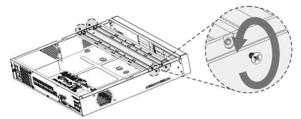
Figure 3-20 Remove screws (2U)
