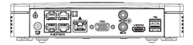
The NVR41-8P-4KS2/NVR41-8P-4KS2/L series rear panel is shown as below.
