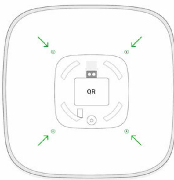
7. Turn the siren over while holding the front and back of the body. Remove the protective plastic panel.
