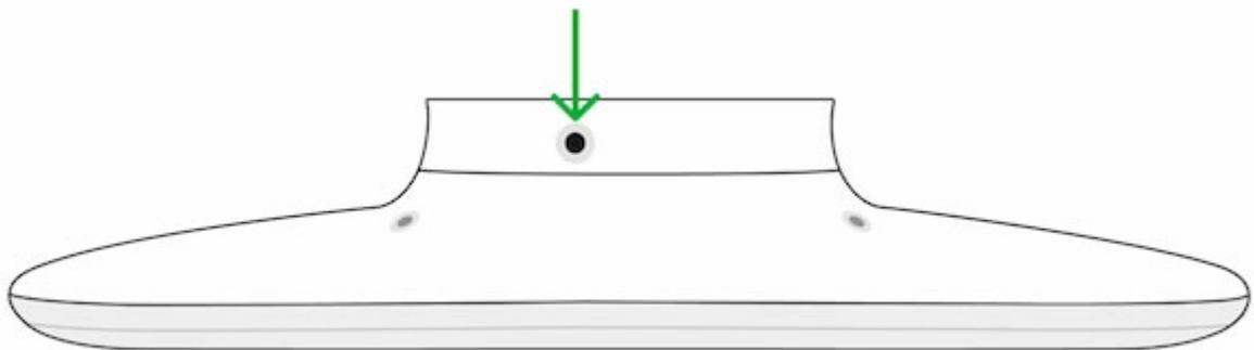
3. Remove the siren from the SmartBracket mounting panel, turning it counterclockwise if the siren is mounted on the mounting plate.
