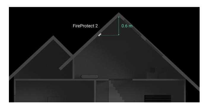
We do not recommend mounting the detector on a wall. This installation is acceptable if closely spaced beams or other obstacles interfere with the installation of the detector. Wall mounting is possible only if the detector is placed at a distance of 15–30 cm below the ceiling but above the doorways.
