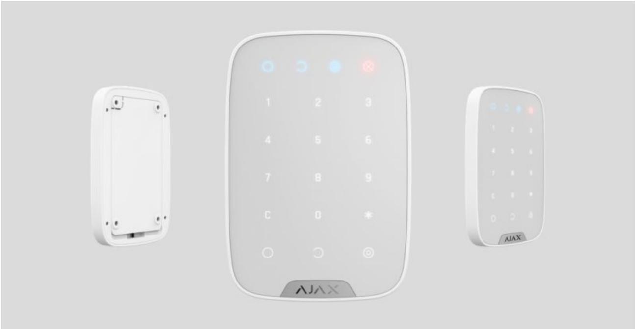
**KeyPad** is a wireless indoor touch-sensitive keyboard for managing the Ajax security system. Designed for indoor use. With this device, the user can arm and disarm the system and see its security status. KeyPad is protected against attempts to guess the passcode and can raise a silent alarm when the passcode is entered under duress.
