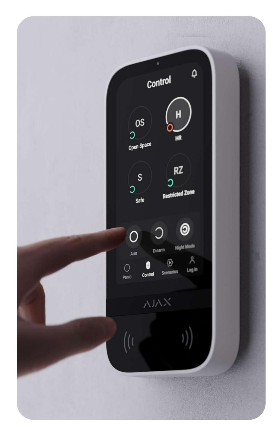
KeyPad TouchScreen supports code types as follows: keypad code (one per keypad) personal code (individual for each user) code for an unregistered person
