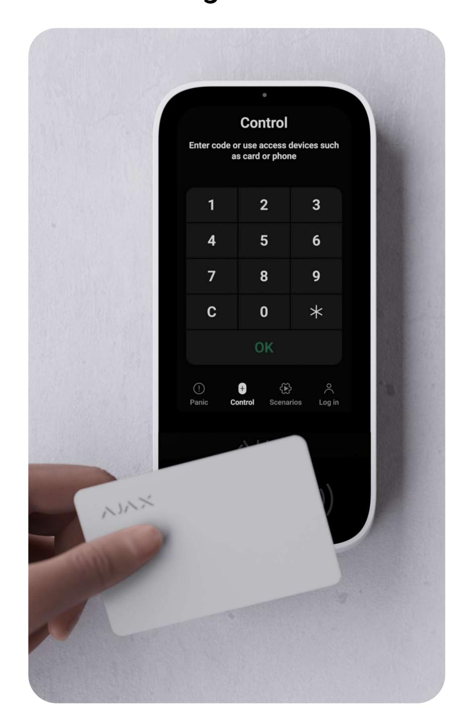
When someone uses the Pass card or the Tag key fob, it's recorded in the event feed of the Ajax apps. The system admin can revoke or restrict the access rights of the contactless access device at any time.
