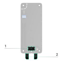
1 - to output the cable through the wall.
