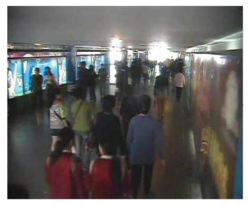
Avoid situations where personnel targets are too large. AcuSense NVRs can analyze target sizes between 1/16 and 1/2 of the image's vertical size. For example, if the camera's resolution is 1080p, the vertical size of the target should be between 64 and 540 pixels.
