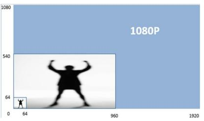
In the following scene, the target takes up almost the whole picture. Adjusting the camera angle so that a targets is detected from a far distance so that it appears a suitable size is suggested.
